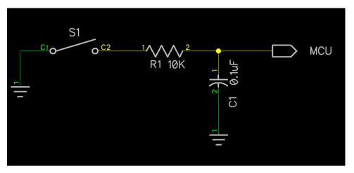
You could enable software debouncing. This causes the firmware to ignore very short pulses. This is enabled with #define ENABLE\_SOFTWARE\_DEBOUNCE in config.h
