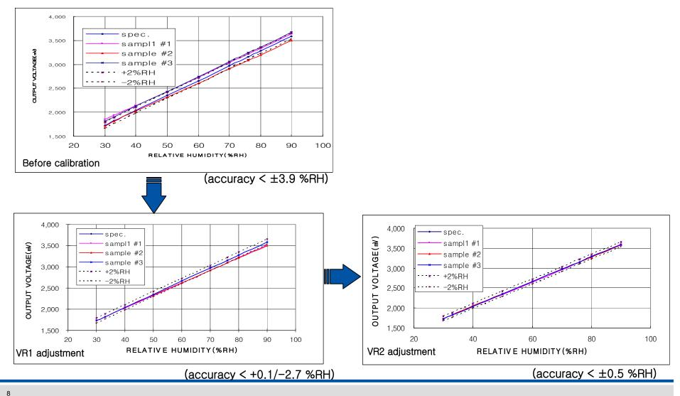
HCH-1000 Series Humidity Sensor Calibration and Output Circuit Data
