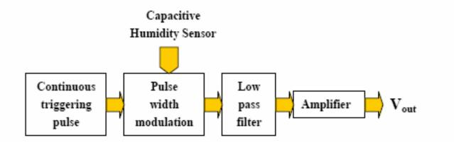
• This sensor support electronic circuitry uses two timers. One timer continuously issues a pulse train in order to trigger the other timer, which operates in PWM mode.
