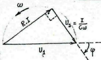
$$\text{On a vu que } \bar{G} = \frac{1}{1+j\alpha} \quad \text{ou} \quad \frac{\bar{U}_2}{\bar{U}_1} = G/\varphi$$
